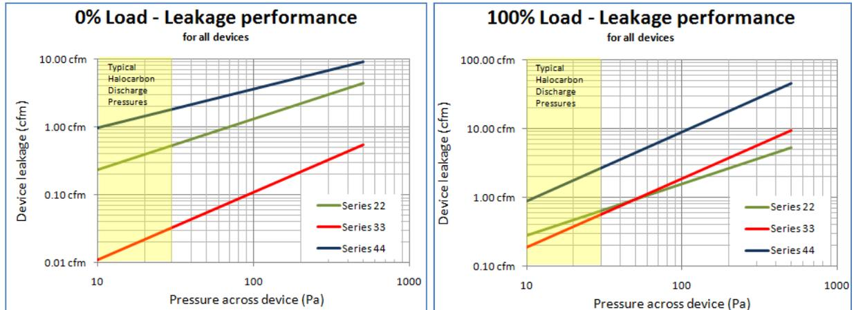
The Series 22 Fire Rated Pathway has two resilient pads that provide an adjustable seal within the raceway. The pads meet in two places to limit leakage. It would take almost 100 empty devices to add the same leakage as around your typical door.
