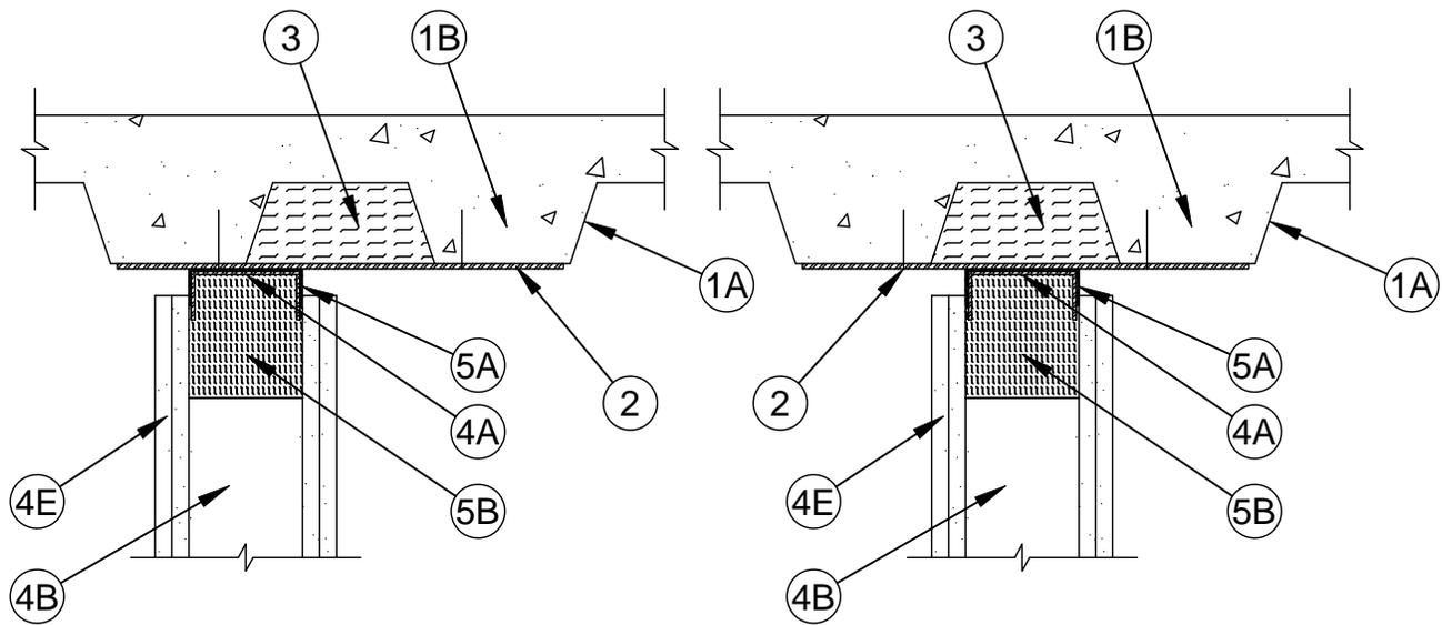
1. **Floor Assembly** - The fire-rated fluted steel floor unit/concrete floor assembly shall be constructed of the materials and in the manner described in the individual Floor-Ceiling Design in the Fire Resistance Directory. The hourly fire rating of the floor assembly shall be equal to or greater than the hourly fire rating of the wall assembly. The floor assembly shall include the following construction features:
