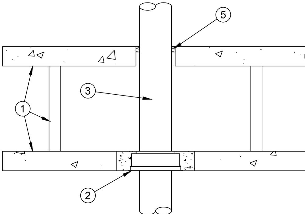
1. **Precast Concrete Units (CFTV)\*** - Precast, pre-stressed, dual deck units constructed in accordance with Floor-Ceiling Design No. K919. At top of floor, diam of opening to be max 1 in. (25 mm) greater than the diam of the penetrant.
