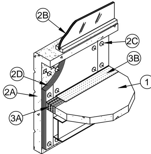
1. **Floor Assembly** - Min 4-1/2 in. (114 mm) thick steel-reinforced lightweight or normal weight (100-150 pcf or 1600-2400 kg/m<sup>3</sup>) structural concrete. Floor assembly to be supported at perimeter edges by spandrel beams having a Restrained or Unrestrained Beam Rating of 2 hr. Edge of concrete floor to be max 8 in. (203 mm) from interior surface of spandrel panel (Item 2A).
