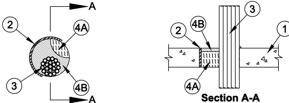
1. **Floor or Wall Assembly** - Min 2-1/2 in. (64 mm) thick reinforced lightweight or normal weight (100-150 pcf or 1600-2400 kg/m<sup>3</sup>) concrete floor or min 3-1/2 in. (89 mm) thick reinforced lightweight or normal weight concrete wall. Floor may also be constructed of any min 6 in. (152 mm) thick UL Classified hollow-core **Precast Concrete Units\***. Wall may also be constructed of any UL Classified **Concrete Blocks\***. Max diam of opening is 6 in. (152 mm).
